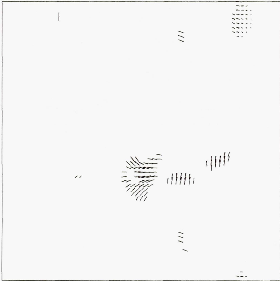
Figure 18.— Two-dimensional slice of the compressive component of the rate of strain (fig. 17) indicated by the arrow in figure 13(a). The structure in the center shows the compressive component aligned perpendicular to the vorticity in figure 15 and parallel to the scalar gradient in figure 16.
