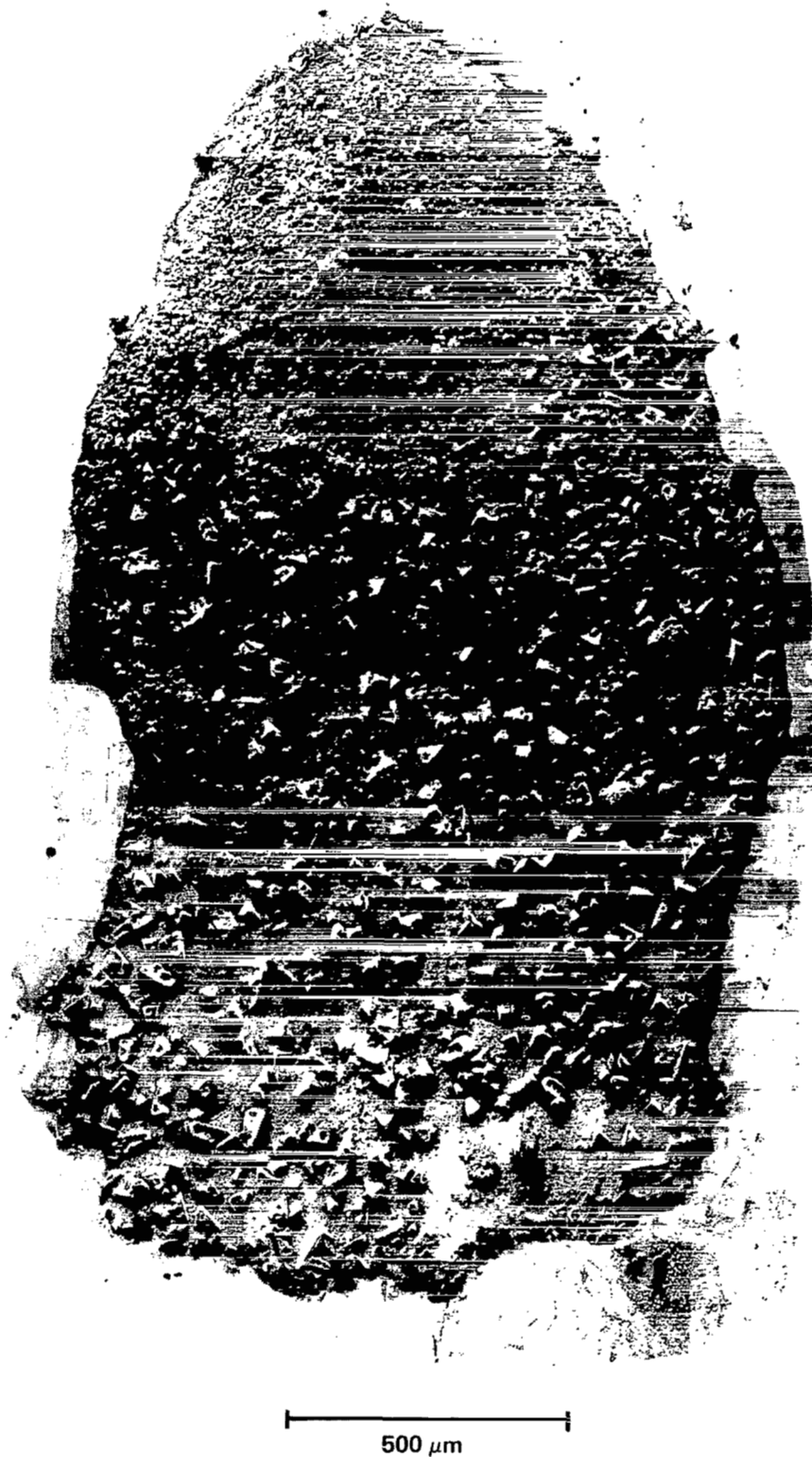
Figure IIb-5. Mosaic electron micrograph of a deposition spot on a plate near the pad perimeter during the STS-4 launch. Spherical particles are \text{Al}_2\text{O}_3 , tetrahedral crystals are copper chloride or a related compound from reaction of HCl with substrate. (Electron microscopy by Alice Dorries)
