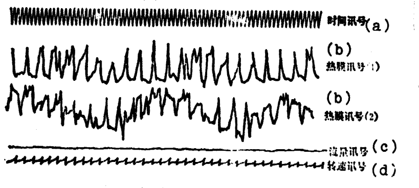
Fig. 7. The oscillograms measured by two hot-wire anemometer probes in the transient process of a rotating stall at n=13,000 rpm: the upper one--the probe located at the root of the blade; the lower one--the probe located at the tip of the blade. Key: (a) Time signals; (b) Hot-wire signals; (c) Flow signals; (d) Signals of rotating speed.
