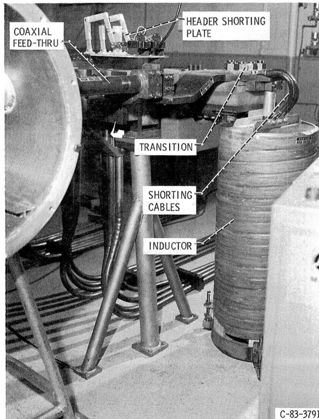
Figure 8. - Atmosphere side of coaxial feed-thru.
