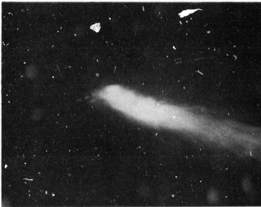
Figure 3-4. Flame Anchoring at U_0 = 50 m/s, FR = 4.65
