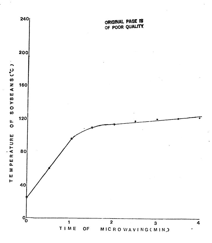
Figure 2: Effect of Microwaving on Temperature of Soybeans at 9.1% moisture.
