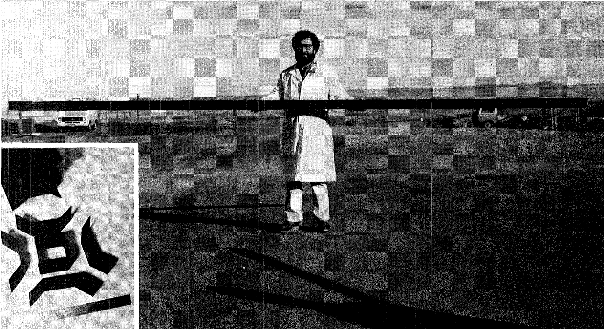
Figure 3-15 Graphite/Epoxy Vertical Member
