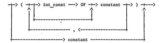
The value part associates a constant with a previously declared variable which is in ROM. The value is placed into ROM with the program thereby defining the variable. This is the only way to assign a value to a variable in ROM. No executable code is generated for a value part.
