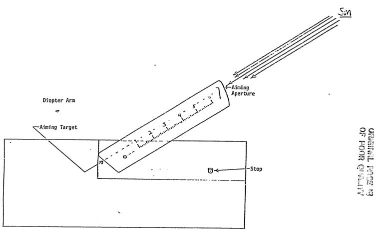
Hold the photometer level by means of Bubble Level; raise arm so that sun spot falls on the aiming target. Read intersection of top of side plate and the scale on the diopter arm. In this example, it reads 1.75.
