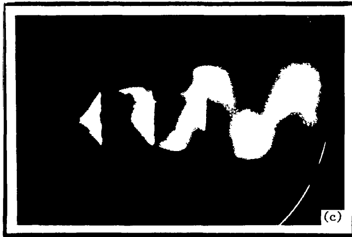
Figure 4.10 Ensemble averaged flow visualization of the supersonic jet at various pressure ratios, PR. PR: (a) 2.035, (b) 2.197 and (c) 2.620.
