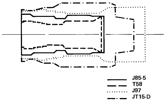
Figure 87. Relative engine sizes of small gas turbines (Ref. 4).
