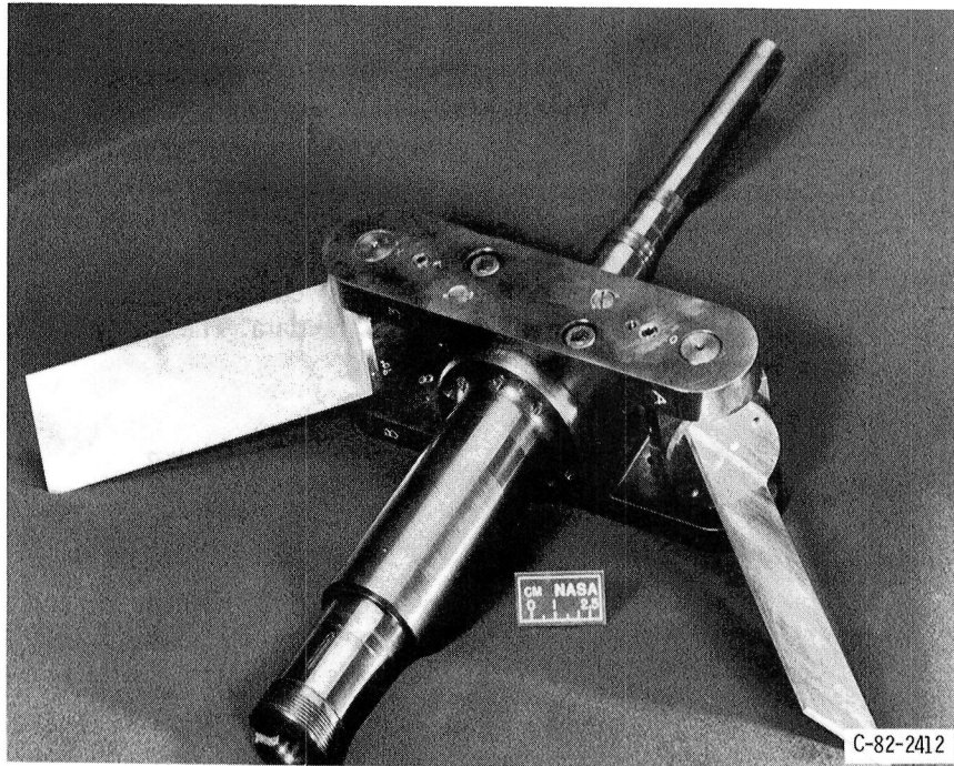
Figure 24. – Two-blade rotor with adjustable sweep and setting angles.
