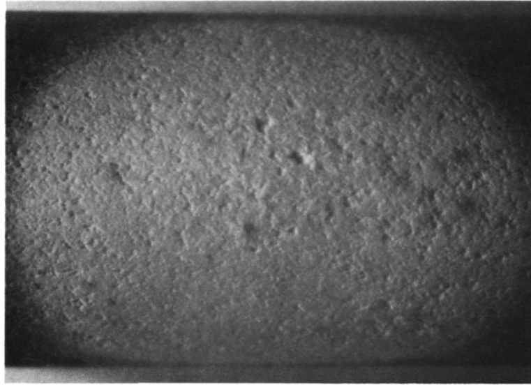
Figure 6. - Smoothed ArO 2 -8% Y 2 O 3 specimen after 100 2.5 second cycles (case D) in a 30 kW plasma flame.
