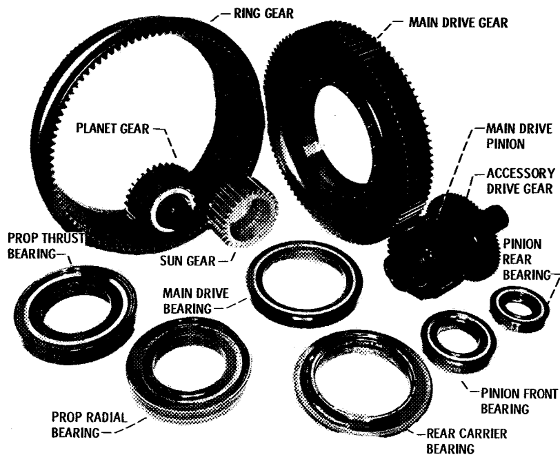
Figure 7. - T56/501 gears and bearings.
