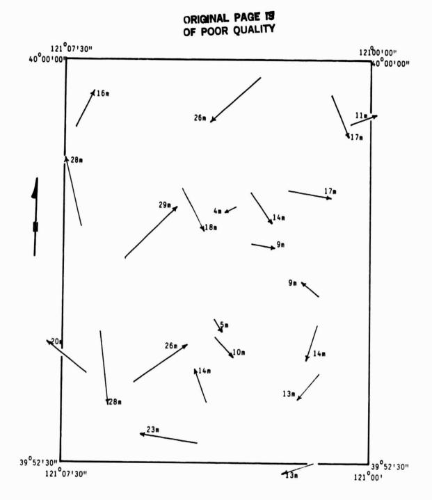
Figure 2.1. Residual vectors for 22 test points. These vectors were calculated by applying first order regressions determined from 20 control points located throughout a 7½ minute quadrangle. Note: the residual vectors are not drawn to scale with respect to the 7½ minute quadrangle.
