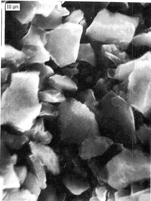
Figure 6.—Structure of typical SiC p /6061 Al composite (top surface).
