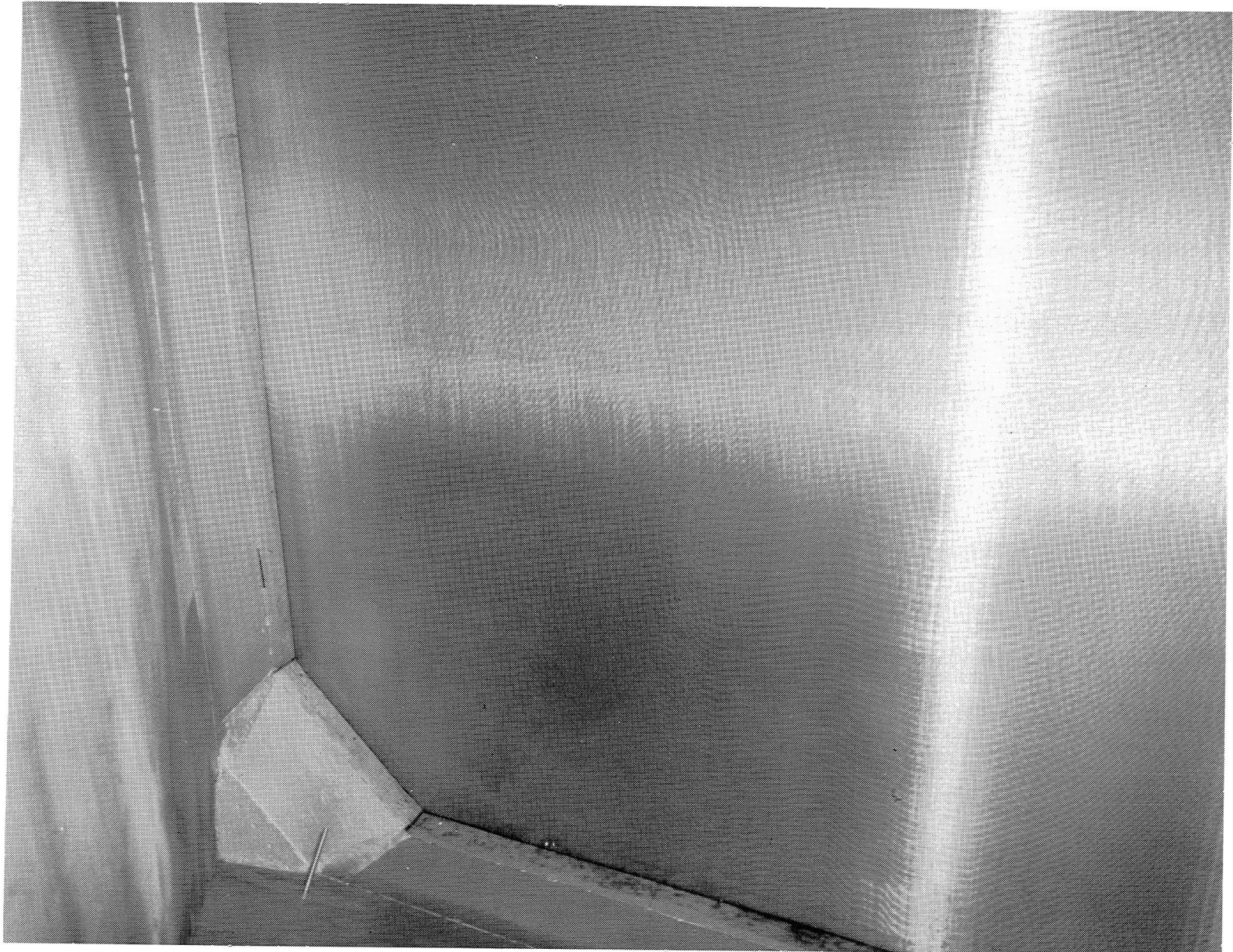
Figure 6.- Photograph of new turbulence-reducing screen installation in Langley Low-Turbulence Pressure Tunnel.
