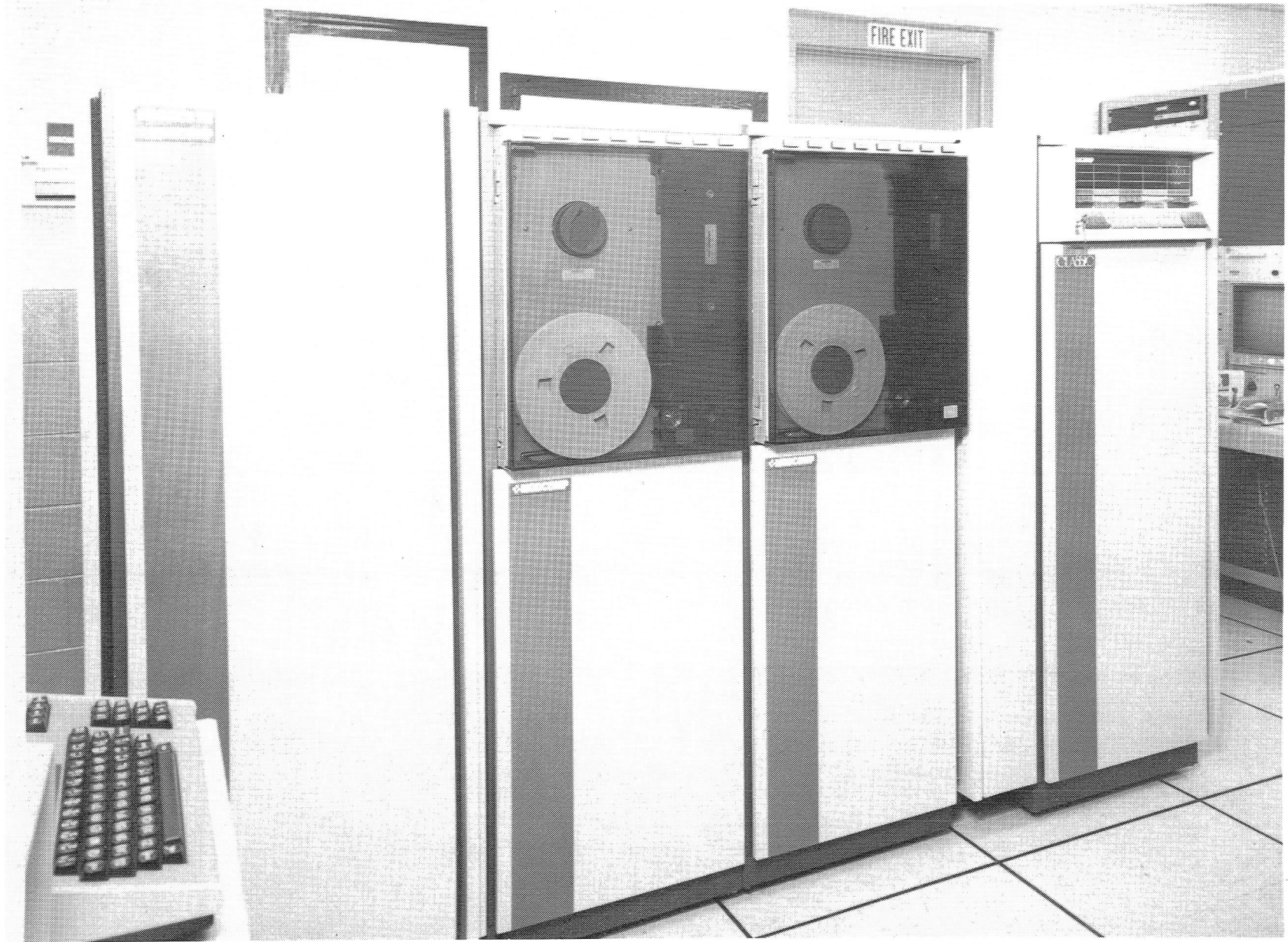
Figure 15.- Photograph of computer and magnetic tape units for tunnel data-acquisition system.
