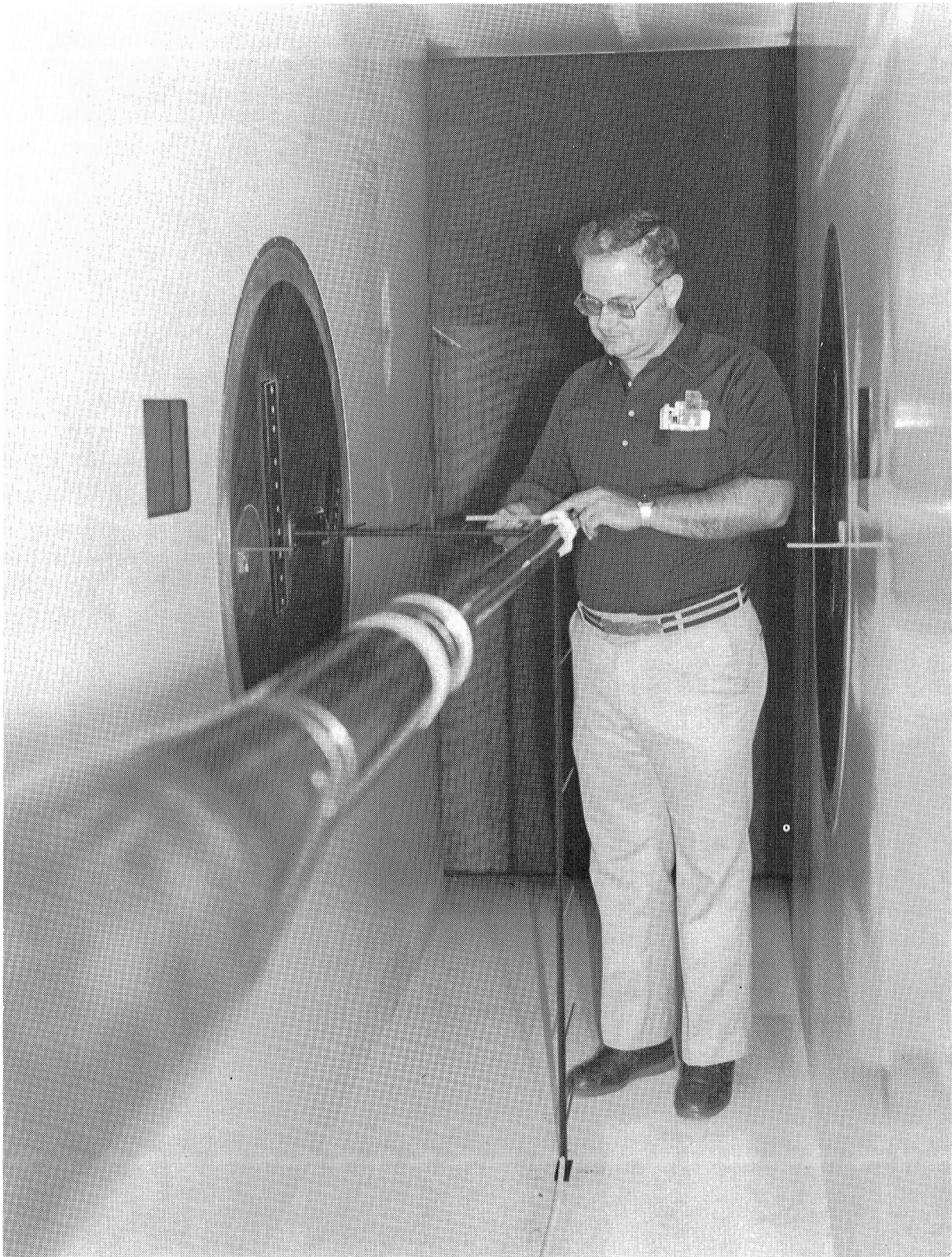
Figure 22.- Photograph of vertical and horizontal rakes of standard pitot-static probes mounted in wind tunnel.
