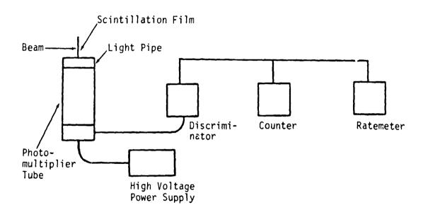
Figure 3. Flux Measurement System
