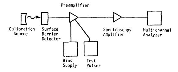
Figure 2. Energy Measurement System
