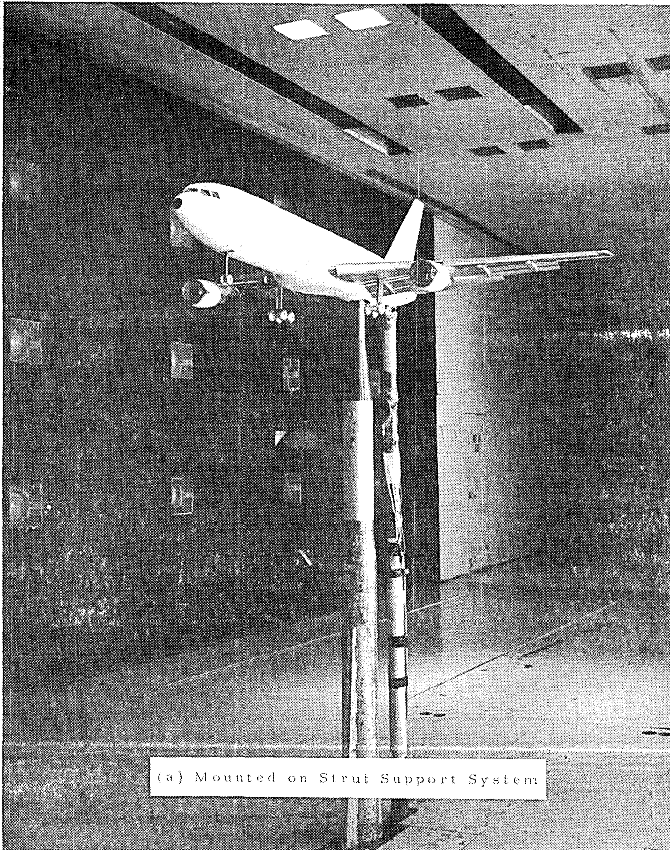
Figure 5. - Photographs of model in Langley V/STOL Tunnel.
