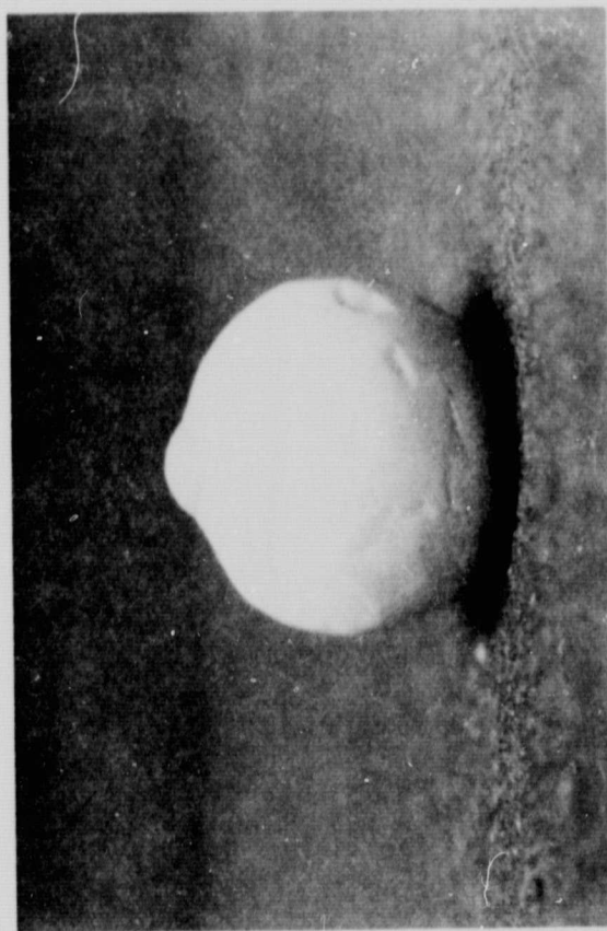
Figure 2. 39.3 \text{Ga}_2\text{O}_3 -35.7 \text{CaO} -25 \text{SiO}_2 , mol%, devitrified glass sample with colored spot (#4) used in MEA/A-1, STS-7.
