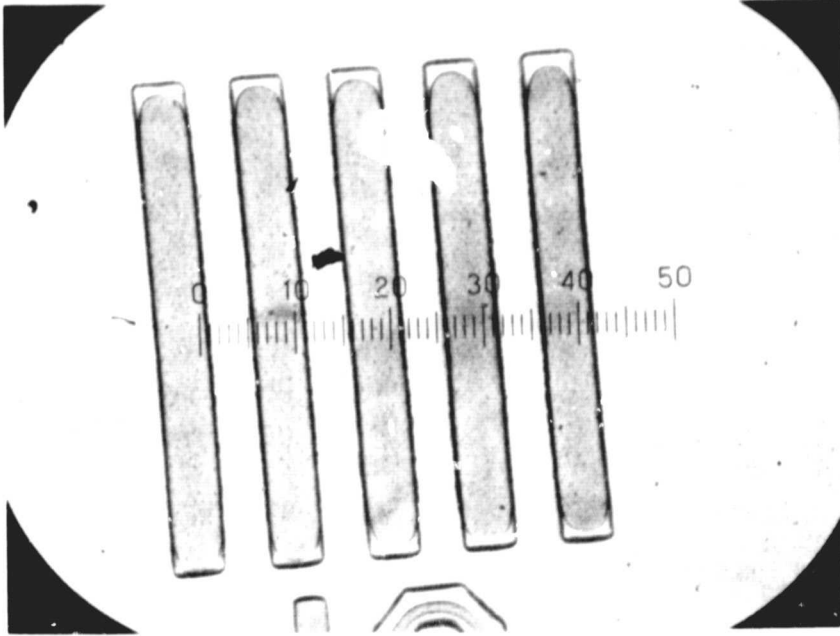
Figure 40. Photomicrograph illustrating the polyimide undercut resulting from over-developing the composite photoresist/polyimide layer. The width of each bar is 0.5 mils or 12.5 microns.
