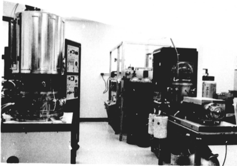
Figure 16. Metallization deposition equipment
