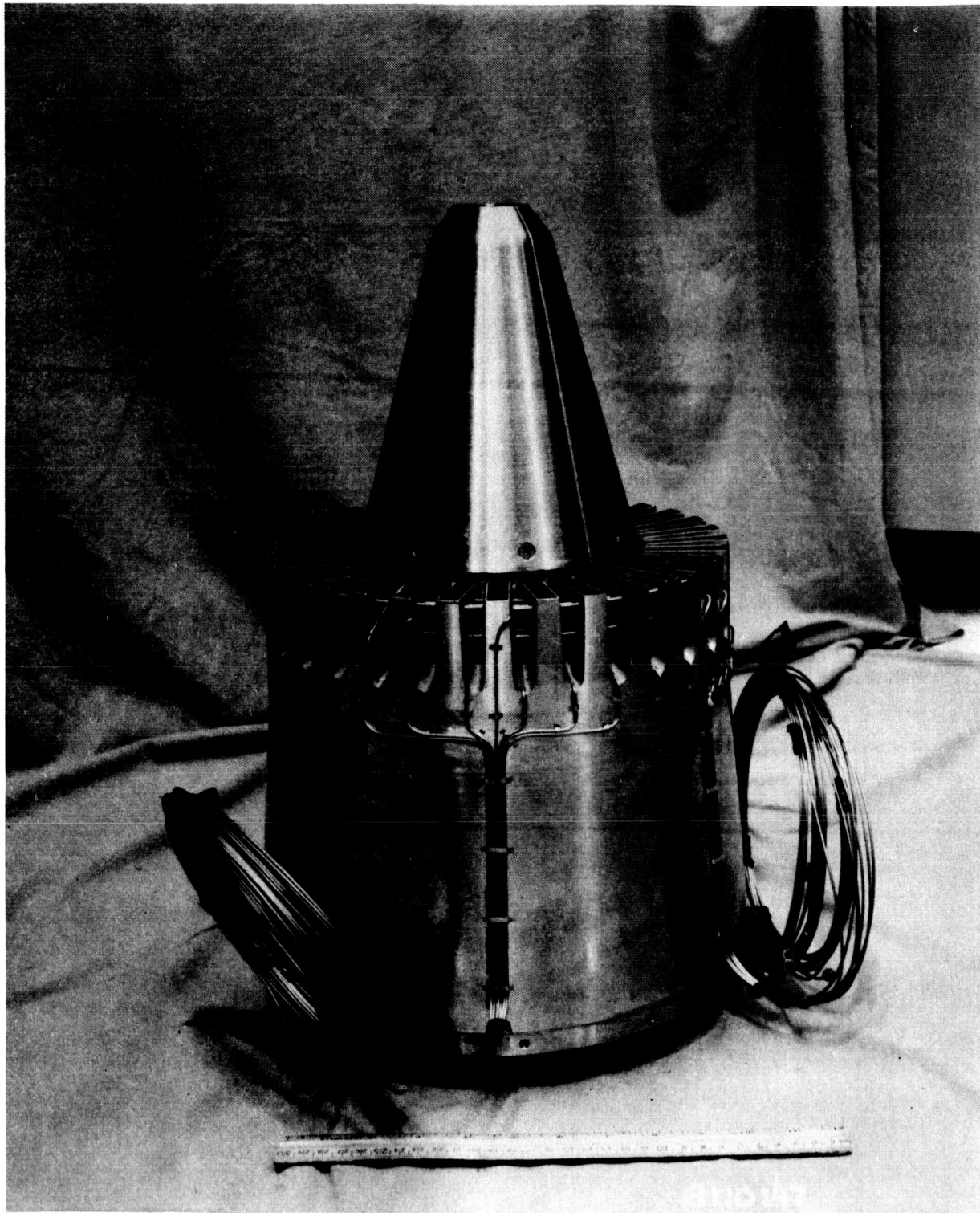
FIGURE 3.2. 32 CHUTE TURBOJET SUPPRESSOR WITH STATIC PRESSURE INSTRUMENTATION FOR BASE PRESSURE MEASUREMENT.
