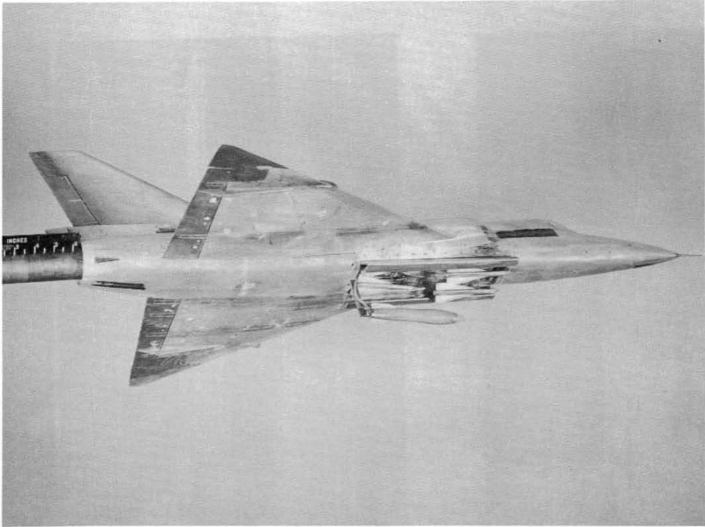
Figure 7.- Convair F-106 wind tunnel model showing stores.
