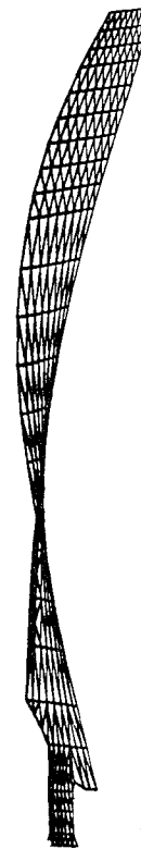
(b) SR3 turboprop finite element model.
