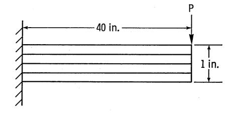
Fig. 3. - Cantilevered laminated beam.
