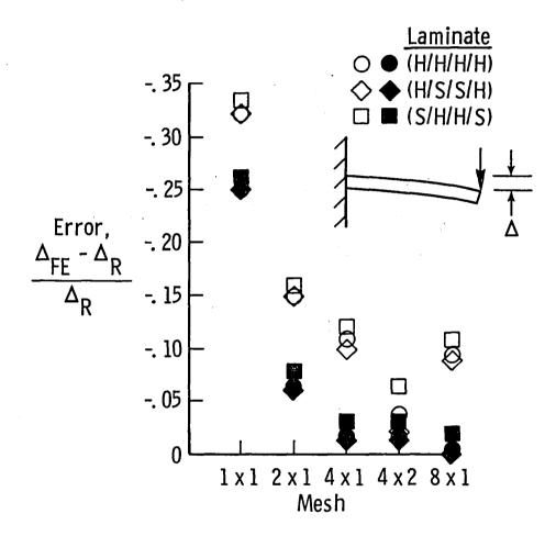
Fig. 5. - Accuracy of calculated tip displacement for tip loaded cantilevered beam. Open symbols are for unmodified RLC element. Solid symbols are for modified RLC element.
