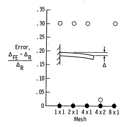
Fig. 6. - Accuracy of calculated tip displacement for thermal loading of unsymmetric cantilevered beam. Open symbols are for unmodified RLC element. Solid symbols are for modified RLC element. (Laminate = (H/H/I/I))
