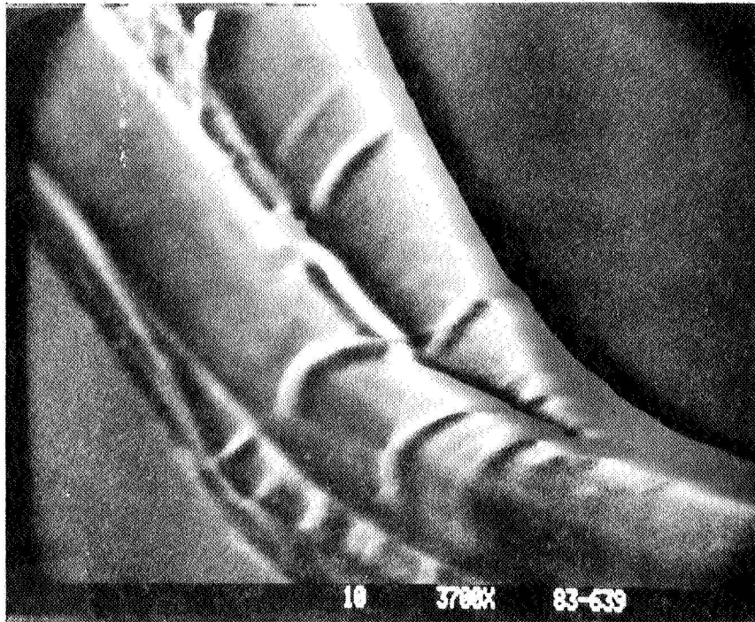
Figure 12. Kevlar fibers (3700X)
