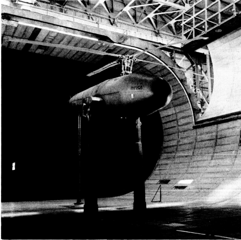
Figure 1. BO-105 rotor system on Ames Rotor Test Apparatus in 40- by 80-Foot Wind Tunnel test section.
