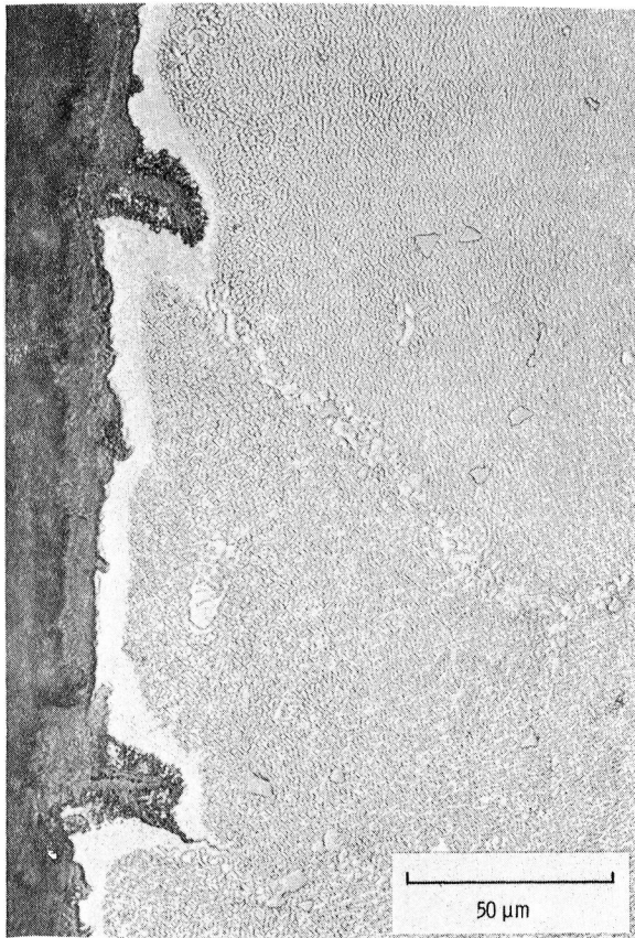
(a) Specimen G27 (compressive strain hold, t_f = 17 hr). Note the crack initiated at the lower grain boundary.
