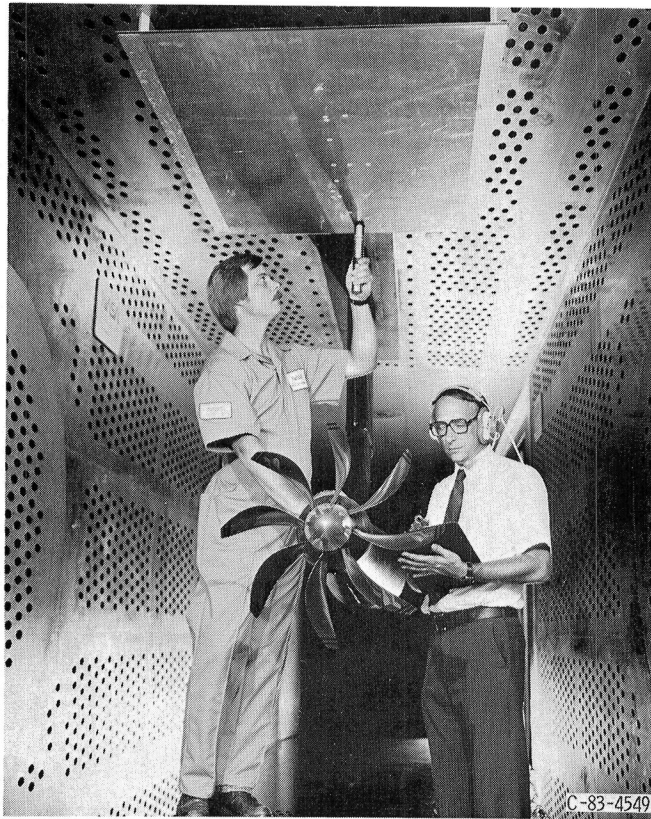
Figure 3. - Plate installed at close to ceiling position.
