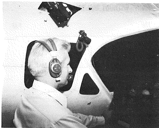
Figure 2. The MH projector in the simulator (above the subject's head).
