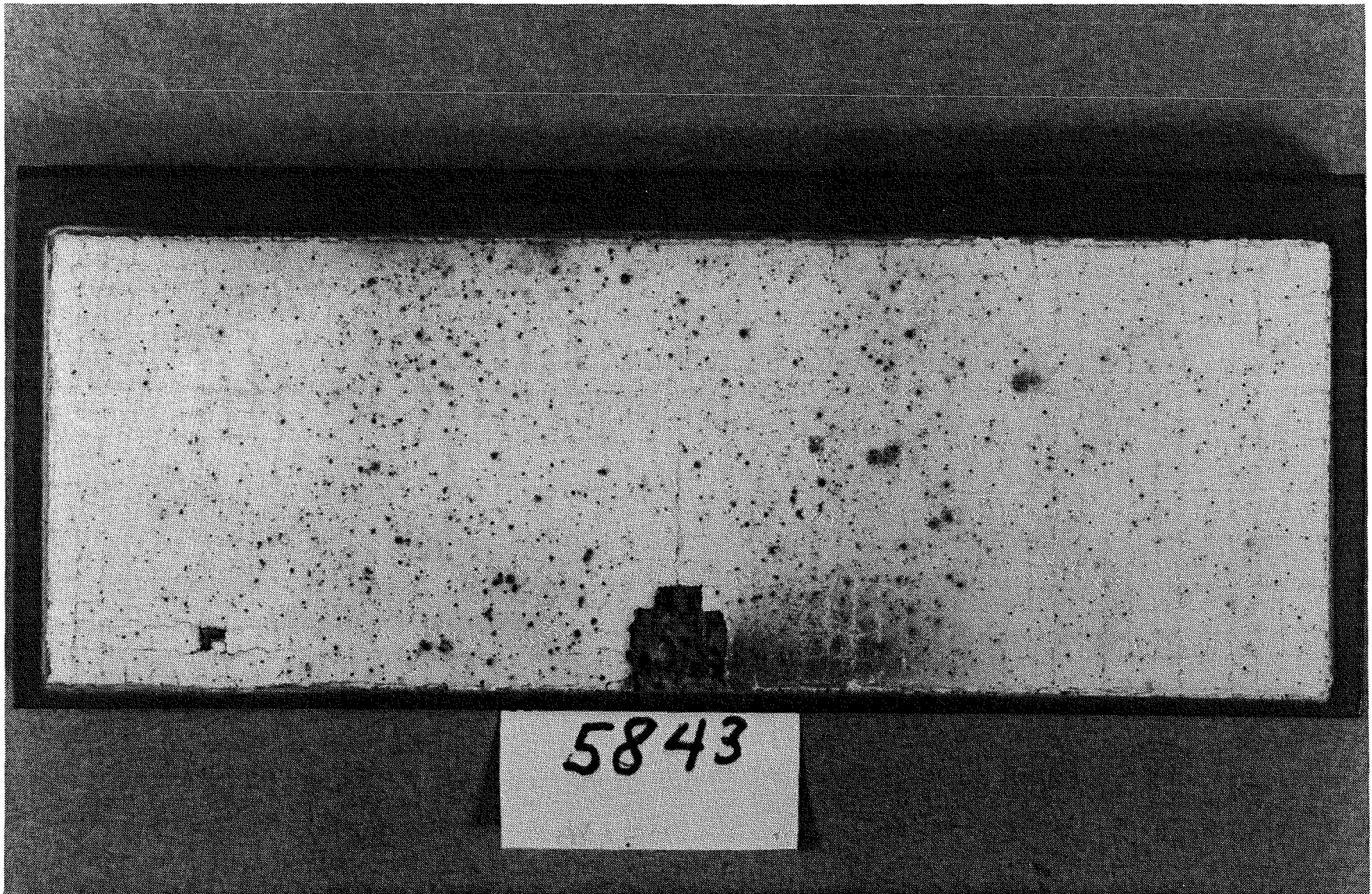
Figure 13. \text{ZrO}_2 - 24 MgO Coated Wire Mesh Shroud Segment After 2689 Thermal Shock Cycles
