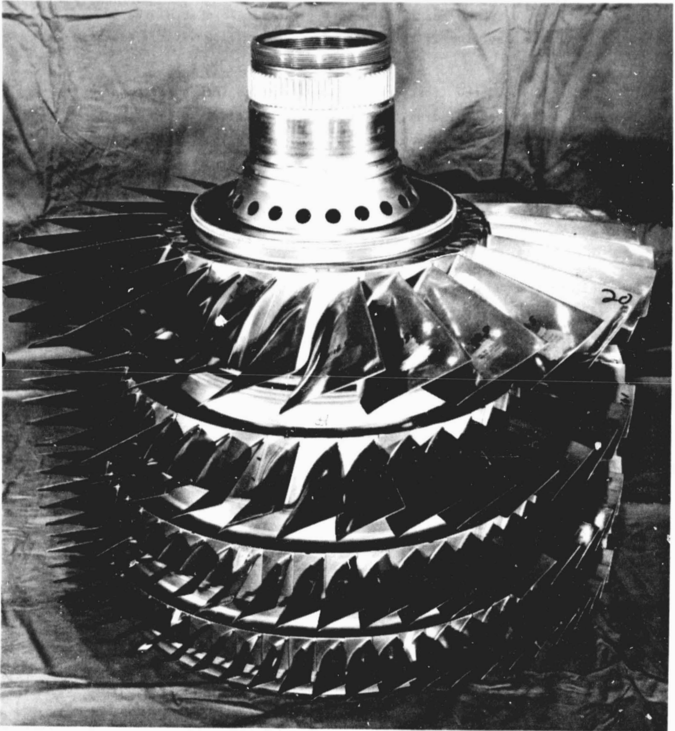
Figure 21. Photograph of First Four Rotor Stages.
