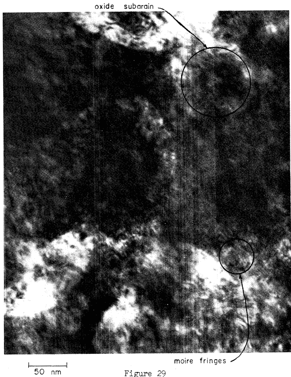
Higher magnification bright field image in just an oxide region of Figure 28a). Possible oxide subgrains and Moire fringes are indicated.
