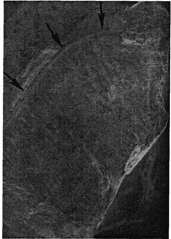
Convex Platform Crack Fracture Surface - Depth Denoted by Arrows (Rest is Lab Break and Saw Cuts).
