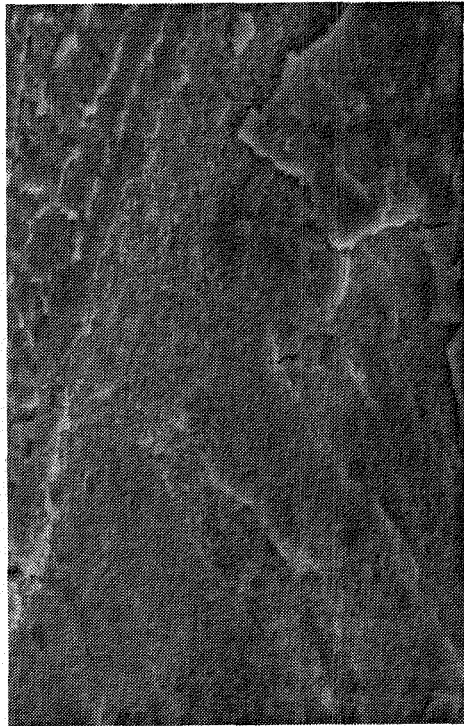
Convex Platform Crack Fracture Surface - Depth Denoted by Arrows (Rest is Lab Break and Saw Cuts).
