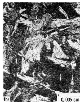
(a) Carburized and hardened case of the CVM AISI 9310 gear showing high carbon fine grain martensitic structure. (b) Core structure of CVM AISI 9310 gear showing low carbon refined austenitic grain size.
