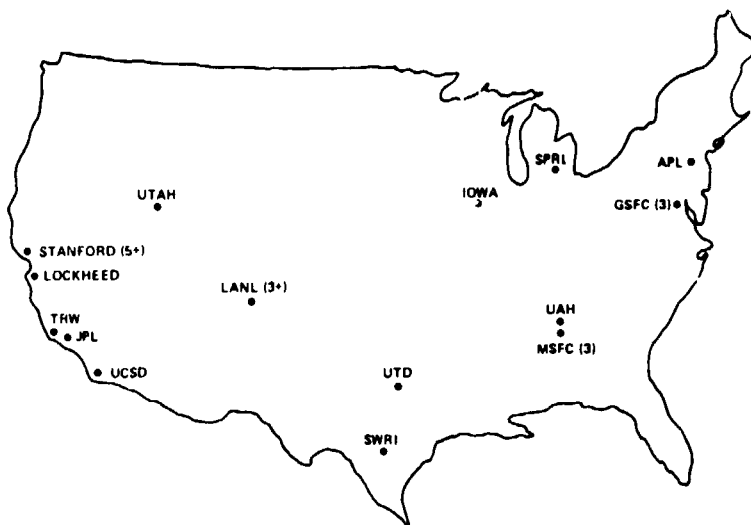
Figure 37. Current SPAN System Nodes. The number of computers linked into a local area network is shown in parentheses.
