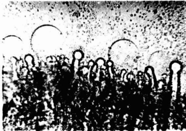
Figure 42. Succinonitrile-Benzene Solid-Liquid Interface. Worm-stalk phase widths are typically less than 10 \mu m for most systems and growth conditions.
