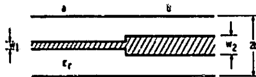
Figure 8. - Top view of a discontinuity in the strip width on a microstrip.
