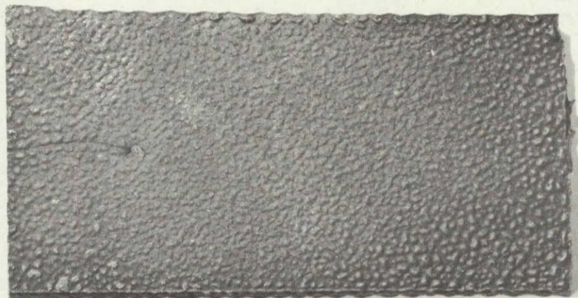
PLV 10059 (Sheet) After 352 Hours in \sim 100\% \text{H}_3\text{PO}_4
