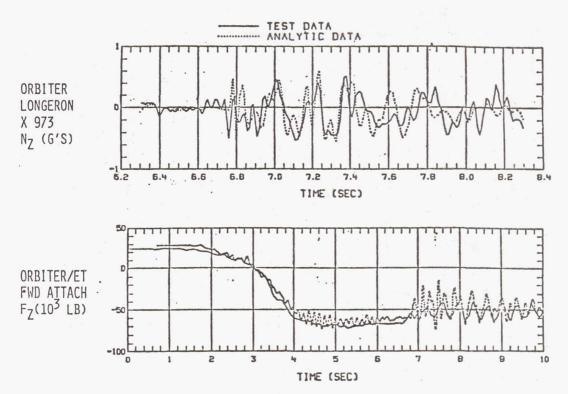
FIGURE 11.- STS-2 LIFT-OFF MEASURED LOADS VERSUS RECONSTRUCTION.
