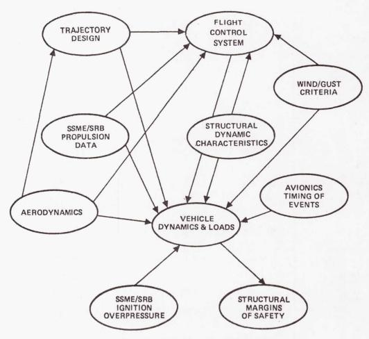
FIGURE 1.- VEHICLE SYSTEMS AND ENVIRONMENT INTERACTIONS.
