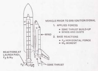
FIGURE 3.- LIFT-OFF CONFIGURATION AND APPLIED FORCES.
