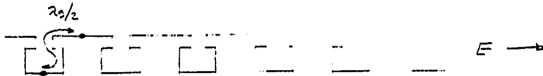
(e) Franklin Antenna (Vertical Polarization Did Not Work)
