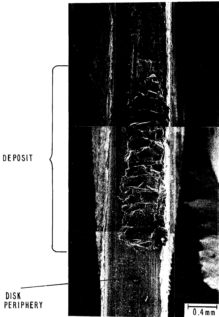
FIGURE 4-9. PHOTOGRAPH OF PERIPHERY OF DISK SHOWING DEPOSIT OF YSZ (TEST TIYZ03)
