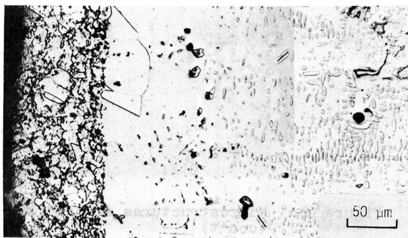
Figure 12. Microstructures of oxidized LPPC substrates (con't) c) LPPC substrate F at 50 cycles d) LPPC substrate F at 130 cycles e) LPPC substrate F at 250 cycles
