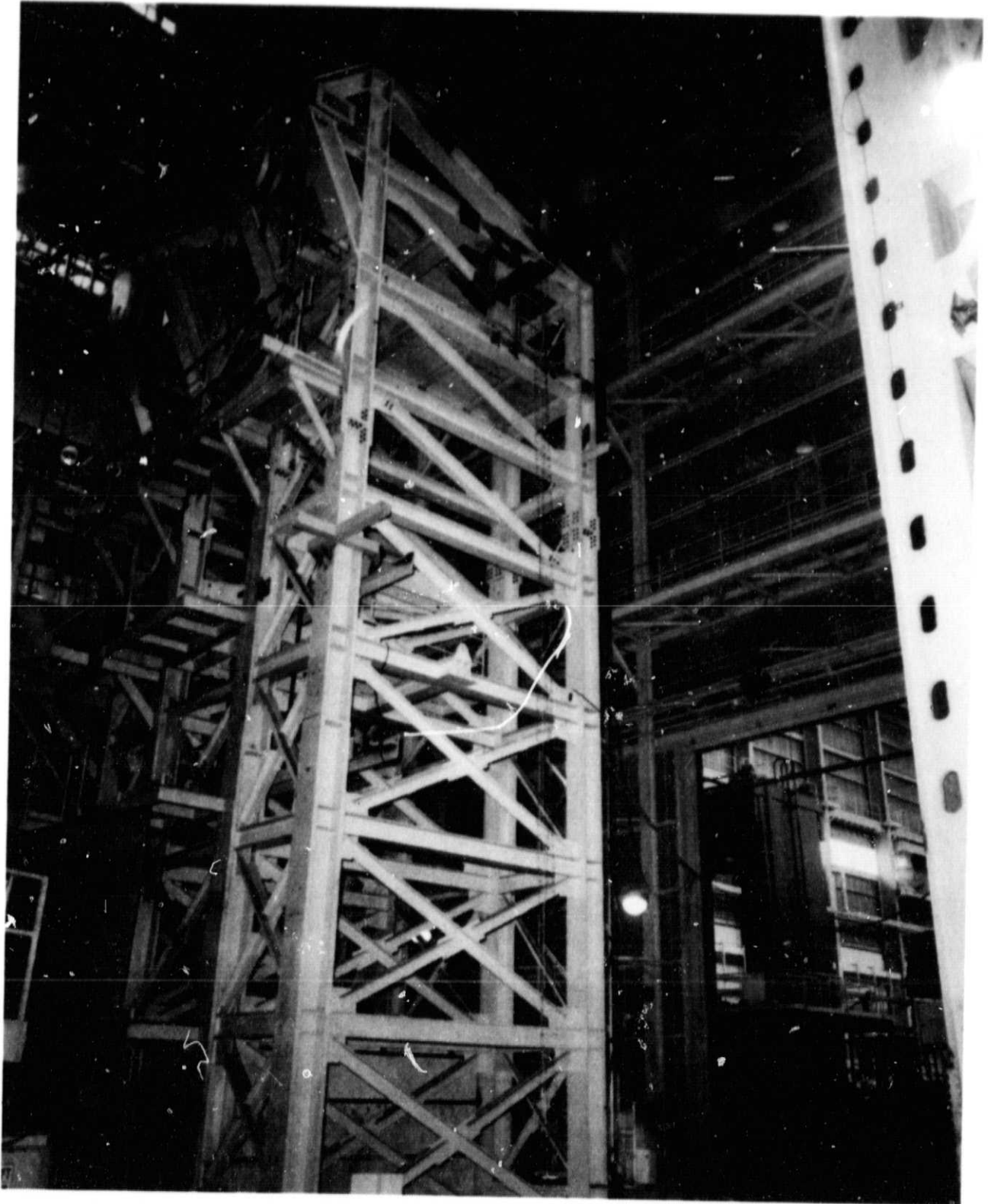
Figure 16. ASTROMAST beam fully deployed in cantilevered modal test configuration.
