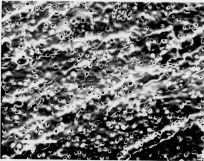
Figure 9. - Platinum-yttria after 100 hr in NH_3 at 1300\text{ }^\circ\text{C} (200X).
