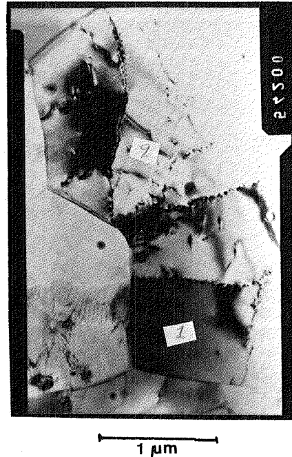
Fig. 9. Transmission Electron Micrograph of As-Extruded Binary Stoichiometric NiAl specimen illustrating the presence of Sub-grain Boundaries.
