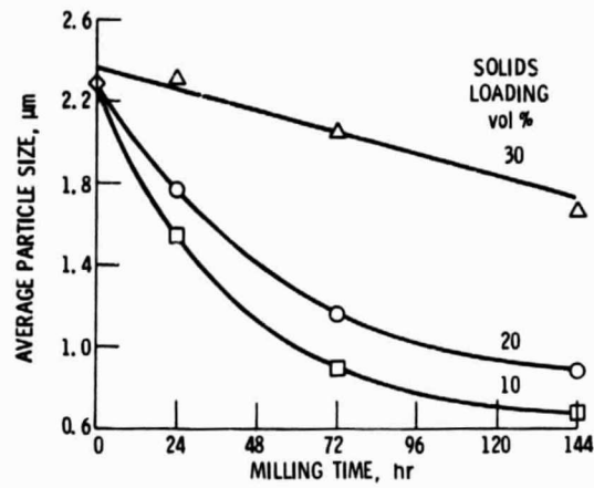
Figure 3. - Effect of milling time on average particle size of SIC for various solids loadings (pH of 9.7, mill speed = 80 rpm).
