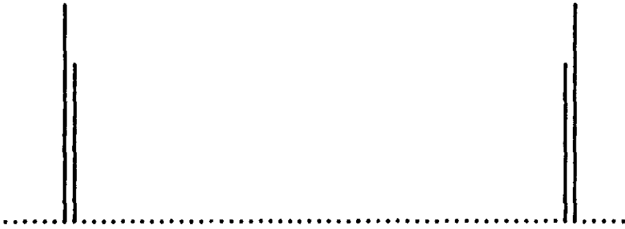
Figure I.2 Band-pass filter sampled desired frequency response as input to a length 64 IFFT.
