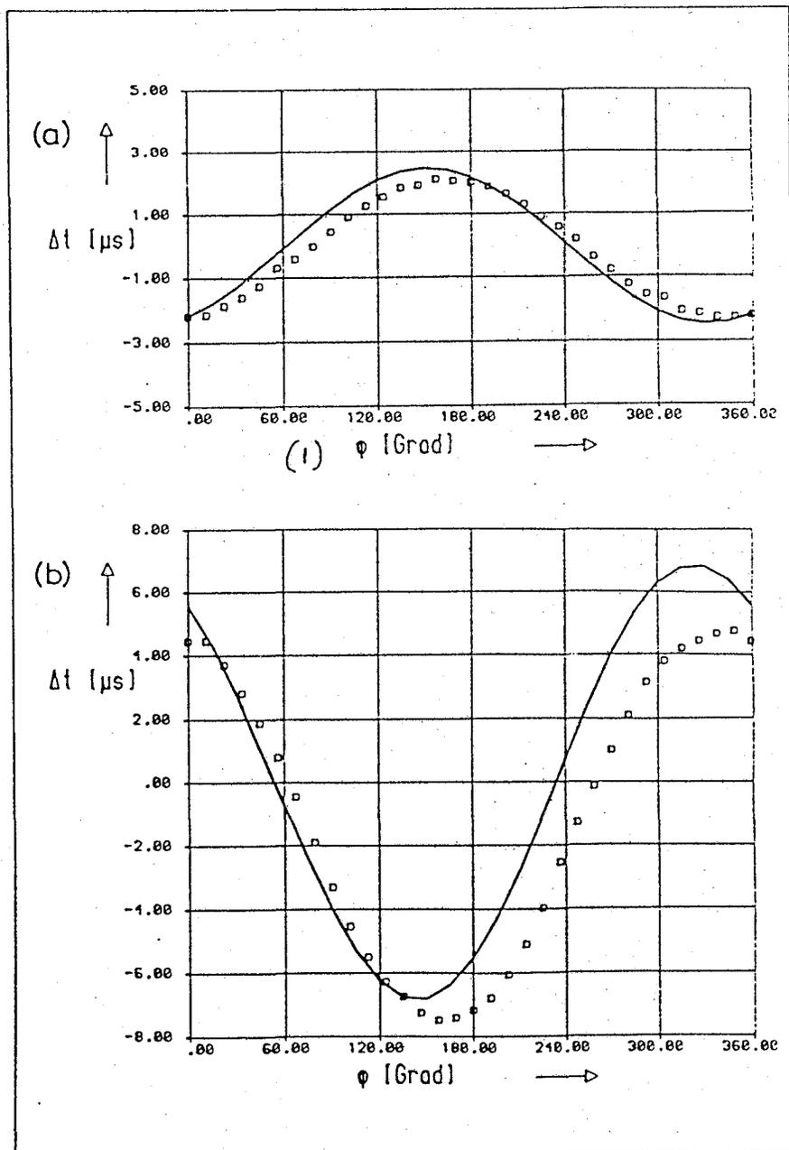
Figure 12: Impulse duration difference in wake outside (a) and inside (b) wake foil, large amplitude  $\Delta\alpha = 8$  degrees; Boundary of linear theory recognizable (solid lines = theory, outlined blocks = experiment) (1) degree
