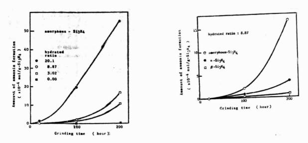
It is understood that there is a tendency for the degree of ammonia formation to increase nearly proportional to the moisture content. Therefore, it is assumed that the ammonia formation reaction in  $\text{Si}_3\text{N}_4$  has a close relation with the water concentration. Furthermore, ammonia was not detected during grinding by purified methanol, and this shows that ammonia formation is not from a reaction which is related to methanol but from the small amount of water which is included.
