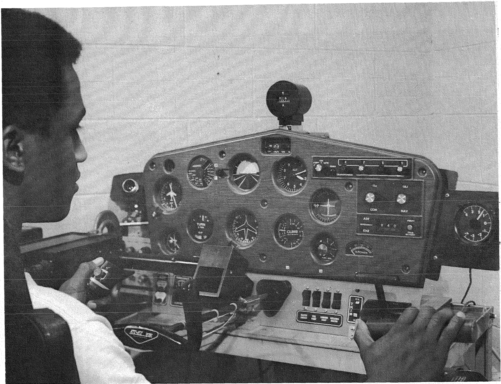
Figure 2.- Test subject flying simulator with round-dial meter side task.
